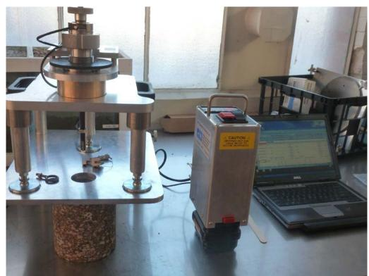
Figure 2. Direct Tension Apparatus
